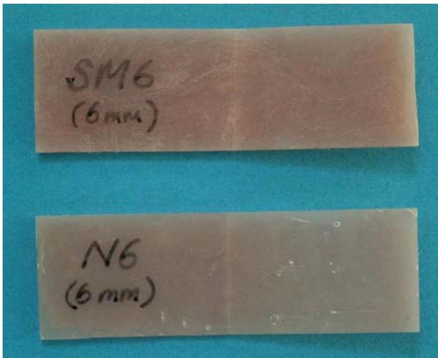
**Fig. 2** Nylon 6,6 and nylon 6 fiber-reinforced specimens after fracture. Specimens remained bound together by fibers across the fracture line
