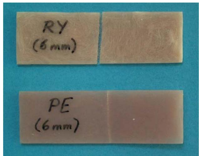
**Fig. 1** Rayon and polyester fiber-reinforced specimens after fracture with fibers holding the sections together
