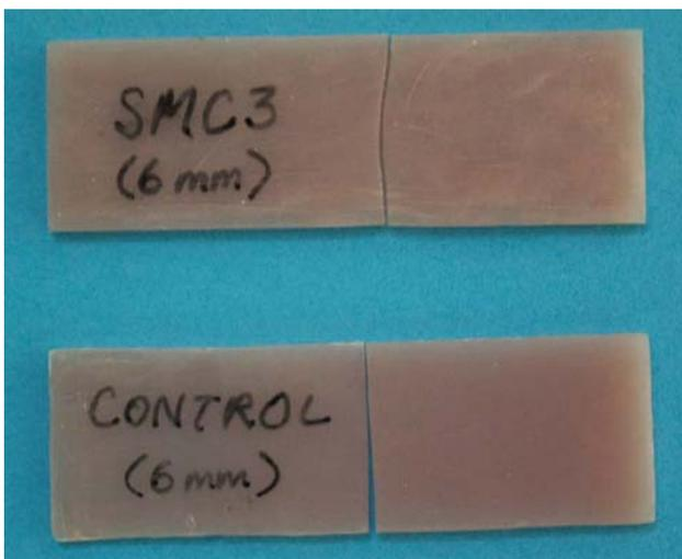
**Fig. 3** Completely fractured specimens reinforced with glass fiber and without fiber
